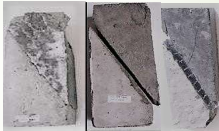
Fig. 4. Failure modes observed in this investigation: mortar failure (left), interface failure (middle), and double failure (right)
