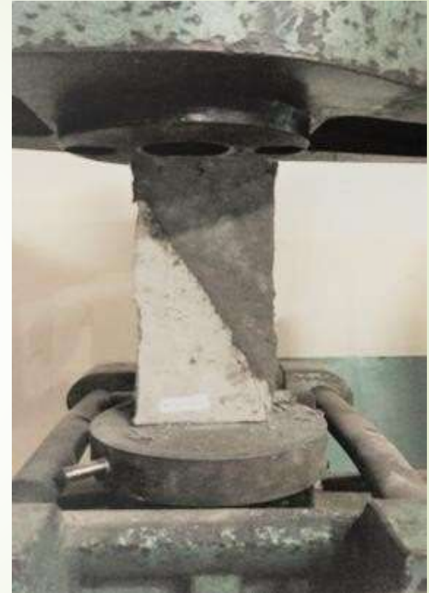
Fig. 2. Composite prism specimen for determining slant shear test under compressive loading
